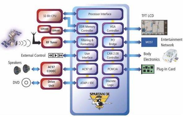
absorb many system functions, including embedded IP cores, custom system interfaces, DSP, and logic. Figure 2-14 below shows such a system.
