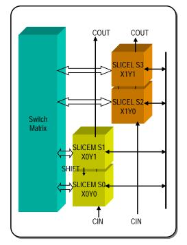
Figure 2-17: Spartan-3 Configurable Logic Block
