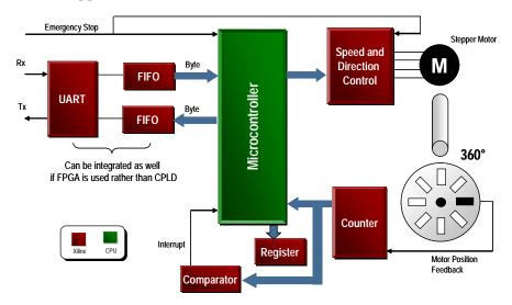
Figure 7-2: Partitioned Design: Microcontroller and CPLD
