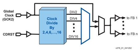
clock nets. The signal is buffered and driven to multiple traces with minimal loading and skew.
