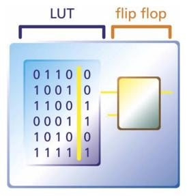
Figure 1-6: SRAM Logic Cell
