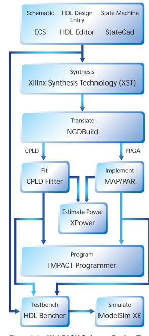
The flow diagram below shows the similarities and differences between CPLD and FPGA software flows.
