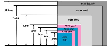
packages are surface mount, with more than half of them ball-grid technologies. The ultratiny packages permit maximum functional capacity in the smallest possible area.
