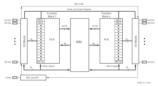
Figure 2-5: CoolRunner-II High-Level Architecture
