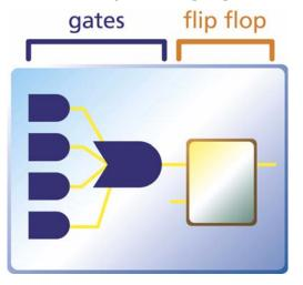
Figure 1-7: OTP Logic Cell
