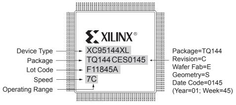
Part marking for non-chip scale package
