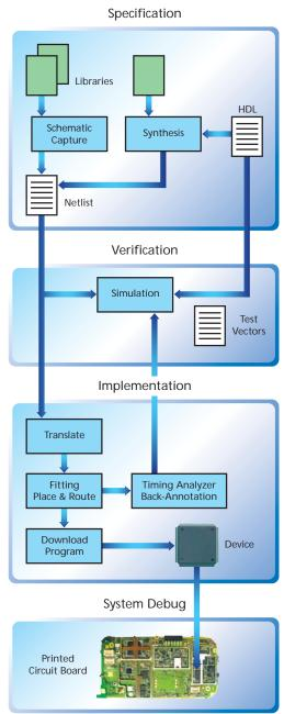
Figure 3-4: The PLD Design Flow
