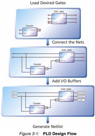
A netlist is a text equivalent of the circuit. It is generated by design tools such as a schematic capture program. The netlist is a compact way for other programs to understand what gates are in the circuit, how they are connected, and the names of the I/O pins.
