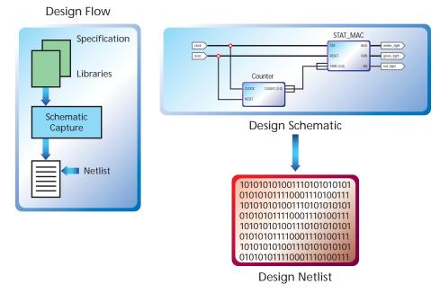
Figure 3-2: Design Specification – Netlist
