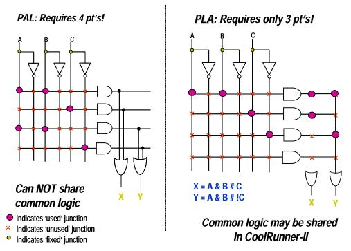
Figure 2-6: Logic Allocation – Typical PAL vs. PLA
