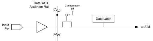
Figure 2-9: DataGATE Function in CoolRunner-II CPLDs
