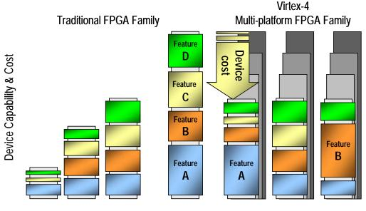
Figure 2-19: Xilinx ASMBL Architecture
