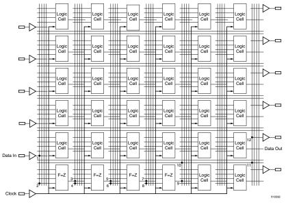
Figure 1-5: FPGA Architecture
