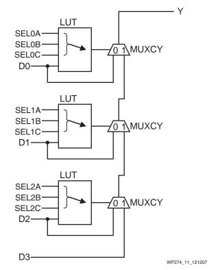
Figure 11: 4-to-1 Multiplexer Using the Carry Chain
