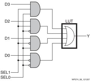
Figure 8: Gates for a 4:1 Multiplexer
