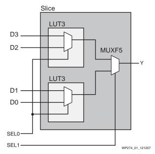
Figure 1: 4:1 Multiplexer Using Dedicated Slice Multiplexer
