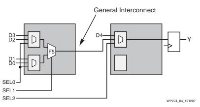
Figure 4: Potential Implementations of 5:1 Multiplexer: Method B
