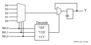
Figure 5: Additional Logic to Support a "When Others" Clause in a Clocked Process
