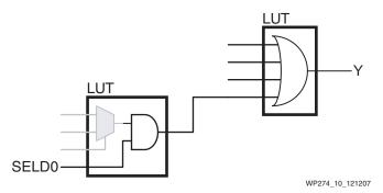
Figure 10: Hiding the Select AND Gate in Other Logic
