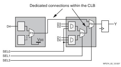
Figure 3: Potential Implementations of 5:1 Multiplexer: Method A
