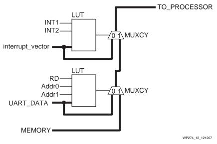
Figure 12: Data Selection to a Processor
