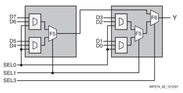
Figure 2: 8:1 Multiplexer Using Two Slices
