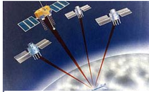
Figure 2 - GPS satellites assisting in position calculation
