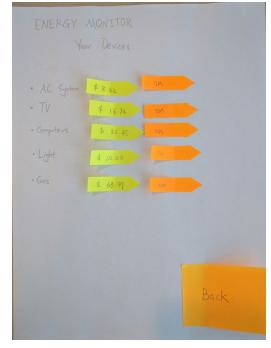
When the design is in home-mode, for all devices it will display the status of the device as well as the cost to power the device for the month.
