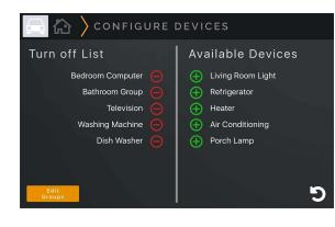
If the user taps on "Configure Selected Devices" on the home screen, the design takes them to this page. Here they can add or remove devices from the list of devices to turn off.
