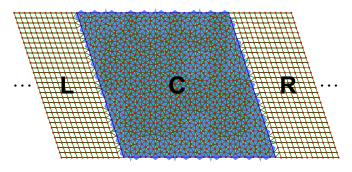
FIG. 11. Schematic illustration of transport simulation setup using the NEGF method. The central part is a finite QL, the left and right parts are two semi-infinite electric leads.
