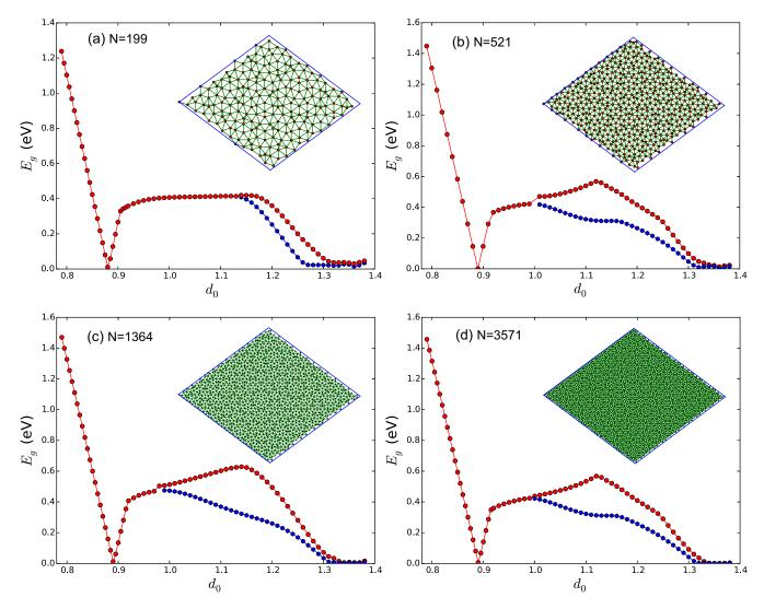
FIG. 9. Energy gap  $E_g$  as a function of interaction strength scale  $d_0$  calculated in quasicrystal approximant containing (a) 199, (b) 512, (c) 1364, and (d) 3571 atoms. The phase transitions among NI, QSH state, and metal occurs in all approximants with different sizes. The dark blue line in the QSH region represents the defect mode in the energy gap.
