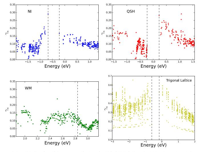
FIG. 10. Participation ratio  $\gamma_n$  of QLs at (a) normal insulator ( $d_0 = 0.86$ ), (b) QSH insulator ( $d_0 = 0.95$ ), and (c) weak metal phases ( $d_0 = 1.34$ ). (d) Participation ratio  $\gamma_n$  of a periodic trigonal lattice.
