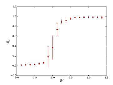
FIG. 4. The spin Bott index as a function of disorder strength W in the disorder Kane-Mele model. The parameters are t=1,  $\lambda_v=1.65t$ ,  $\lambda_{SO}=0.3t$ , and  $\lambda_R=0$  [38]. For each W, 10 samples with 1600 atoms are used to calculate the spin Bott index. A disorder-induced topological phase transition occurs around W=1.0t. This is consistent with the conductance calculation in previous work [38].
