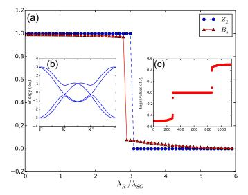
FIG. 3. Topological phase transition in the Kane-Mele model. The parameters are t=1,  $\lambda_v=0.1t$ ,  $\lambda_{SO}=0.06t$  [1]. (a) The  $\mathbb{Z}_2$  invariant and spin Bott index  $B_s$  versus  $\lambda_R/\lambda_{SO}$ . The inset shows the (b) band structure and (c) eigenvalues of  $P_z$  (in units of  $\hbar$ ) upon phase transition with  $\lambda_R/\lambda_{SO}=3$ , where both the band gap of the Hamiltonian and the spectral gap of  $P_z$  almost vanish.
