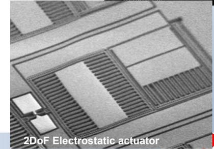
2DoF Electrostatic actuator
