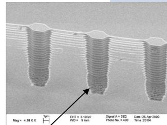
Footing at the bottom of device layer
