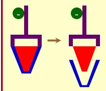
By depositing a metal into or on to a mold or mandrel, a free-standing metal object is made
