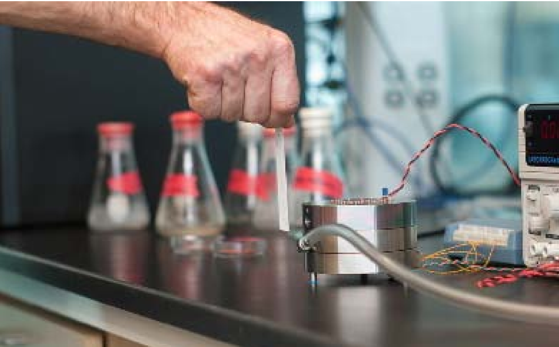
Video of nanofiber sensor response to 10 ug Meth simulant disperse in a filter paper
