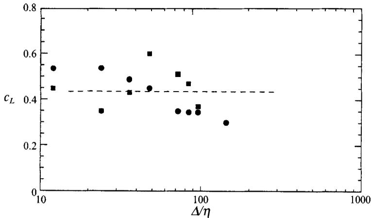
FIGURE 25. Circles: model constant  $c_L$  derived from the balance of SGS energy dissipation for the dissipative similarity model, as function of  $\Delta$  (top-hat filter). Squares: model constant  $c_L^{dyn}$  derived from the dynamic model, based solely on the resolved velocity field.
