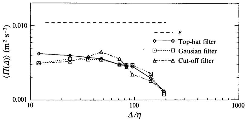
FIGURE 11. Symbols: average subgrid-scale energy flux  $\langle \Pi(\Delta) \rangle$  as function of filter size  $\Delta$ , for the top-hat filter. As a reference, the horizontal dashed line represents the large-scale estimate for the overall rate of dissipation  $\epsilon \approx u'^3/l \sim 0.011 \text{ m}^2/\text{s}^3$ .
