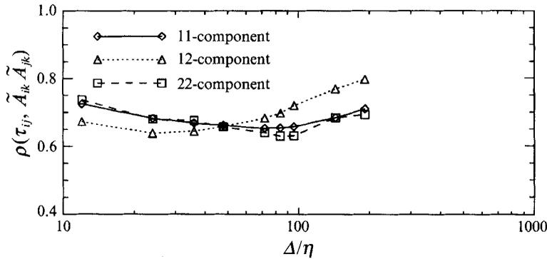
FIGURE 22. Correlation coefficients between  $\tau_{ij}$  and  $\tilde{A}_{ik} \tilde{A}_{jk}$  as function of filter width (using the top-hat filter). The different lines are for different tensor elements.
