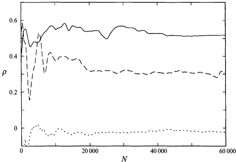
FIGURE 20. Running convergence plot for the correlations between  $L_{11}$  and  $\tau_{11}$  as computed from the turbulence data (solid line), from the random-phase synthetic field, displaying a  $-\frac{5}{3}$  spectrum (dashed line) and white noise (dotted line). A top-hat filter with  $\Delta = 14\delta$  has been used.
